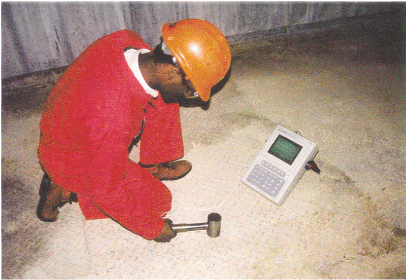
Figure 3. Applying the tap test to chequer plate flooring.
